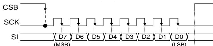
Command data output timing: SCK falling edge operation
