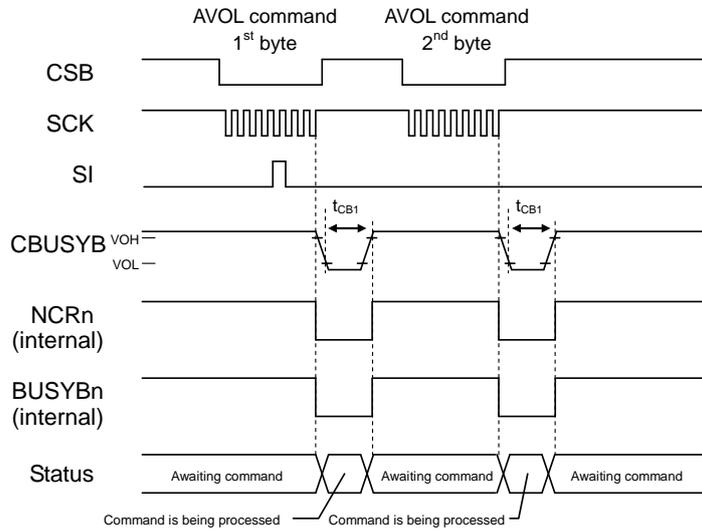
Speaker amplifier volume setting by AVOL commands is valid only when Class AB speaker amplifier is used. When a Class D speaker amplifier is used, the setting value is ignored and +0.0dB is selected.
