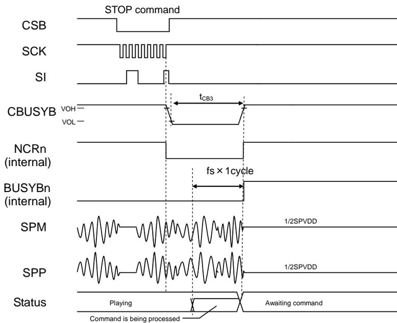
● STOP command (when the FAD bit is "H")
