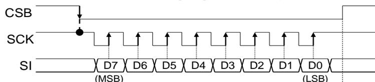
Command data input timing: SCK falling edge operation
