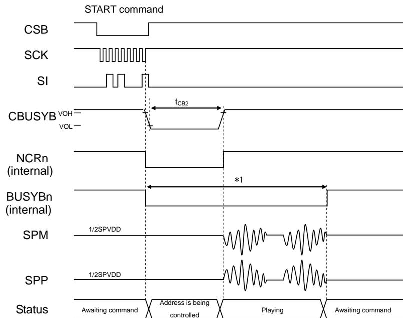
When the START command is input, the address data of the phrase to be played after the command processing time ( $t_{CB2}$ ) is read from the flash memory. When the phrase address data is read, the specified phrase starts playback, and when playback is completed, the BUSYB signal of the playback channel becomes "H" level.
