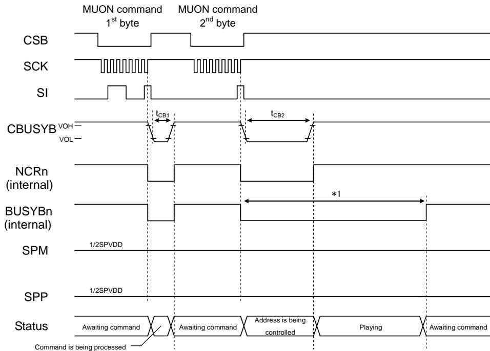
When the first byte of the MUON command is input, the device waits for the input of the second byte after the command processing time ( $t_{CB1}$ ). When the second byte is entered, the silence time is calculated after the command processing time ( $t_{CB2}$ ). When the calculation of the silence duration is completed, the calculated silence is played back, and when the playback is completed, the BUSYB signals of the playback channels become "H" level.
