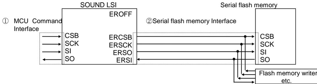
① Rewrite using the clock synchronous serial interface of the MCU command interface
