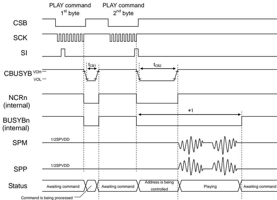
When the first byte of the PLAY command is input, the device waits for the input of the second byte after the command processing time ( $t_{CB1}$ ). When the second byte is entered, the address data of the phrase to be played after the command processing time ( $t_{CB2}$ ) is read from the flash memory.
