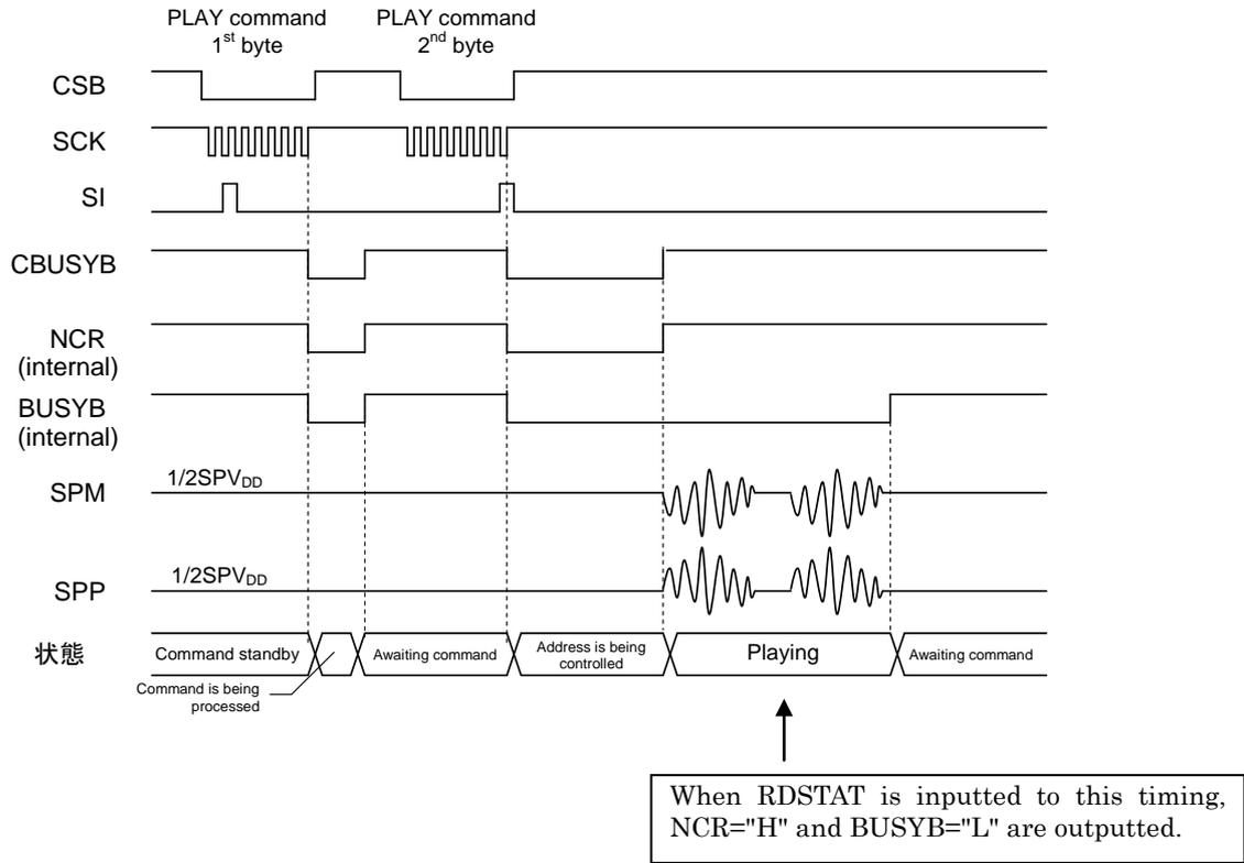
NCR outputs "L" during command processing and address administration, and outputs "H" in other state.
