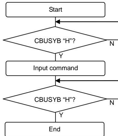
2-Byte Command Input Flow (applied to the AMODE, PLAY, FADR, MUON, CVOL, and AVOL commands)
