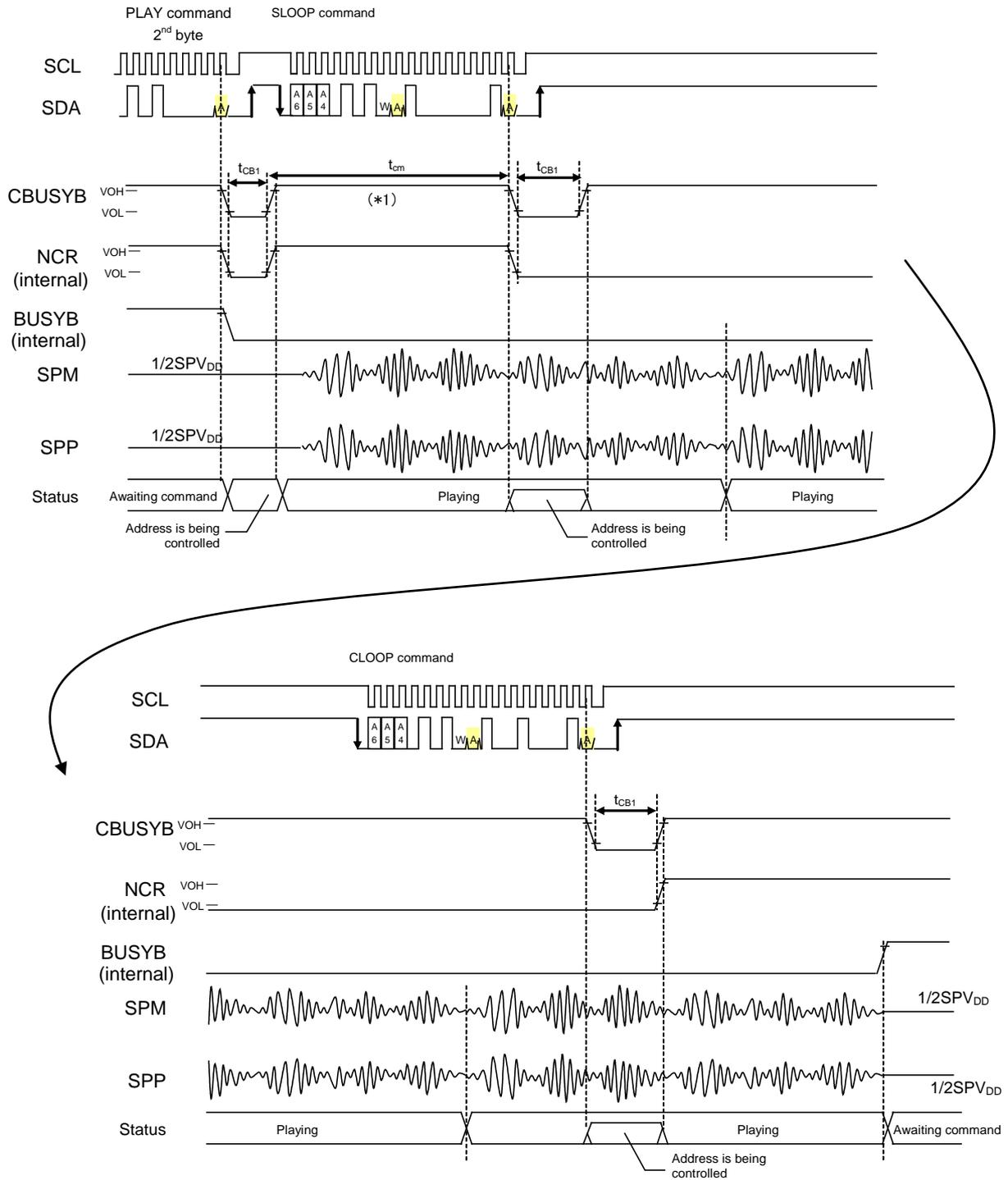
\*1: The SLOOP command must be inputted within  $t_{cm}$ .
