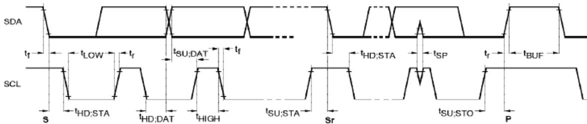
Serial ROM Interface Timing (Applied to both ML22420 and ML22460)
