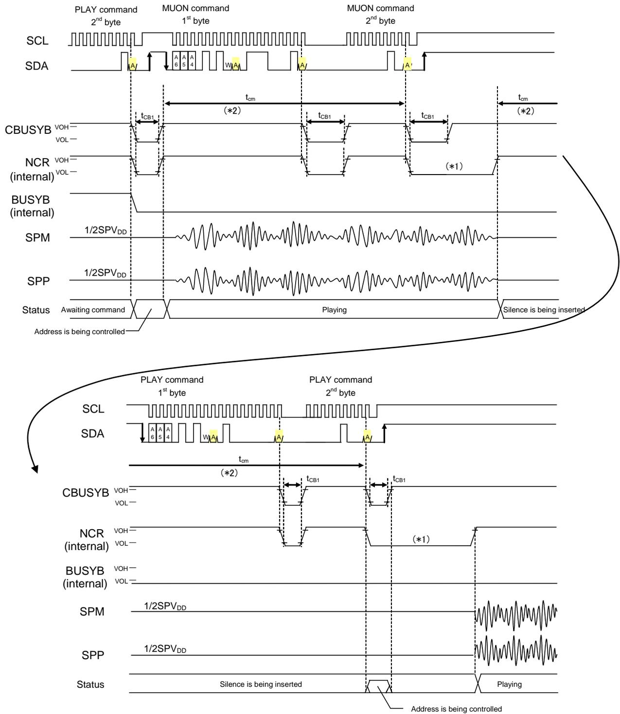
\*1: The time length of “L” level of the NCR signal during playback or silence insertion varies depending on the input timing of command.
