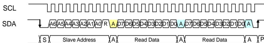
Setting of the slave address using the SAD0 to 2 pins
