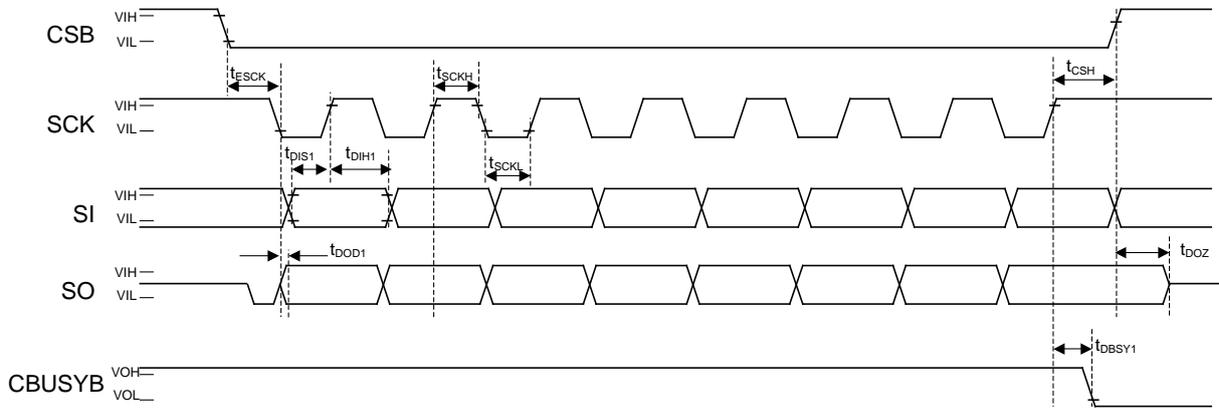
**Serial Command Interface Timing (Applied to ML22420)**
