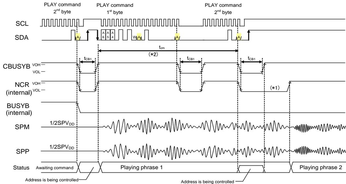
\*1: The time length of “L” level of the NCR signal during playback varies depending on the input timing of command.
