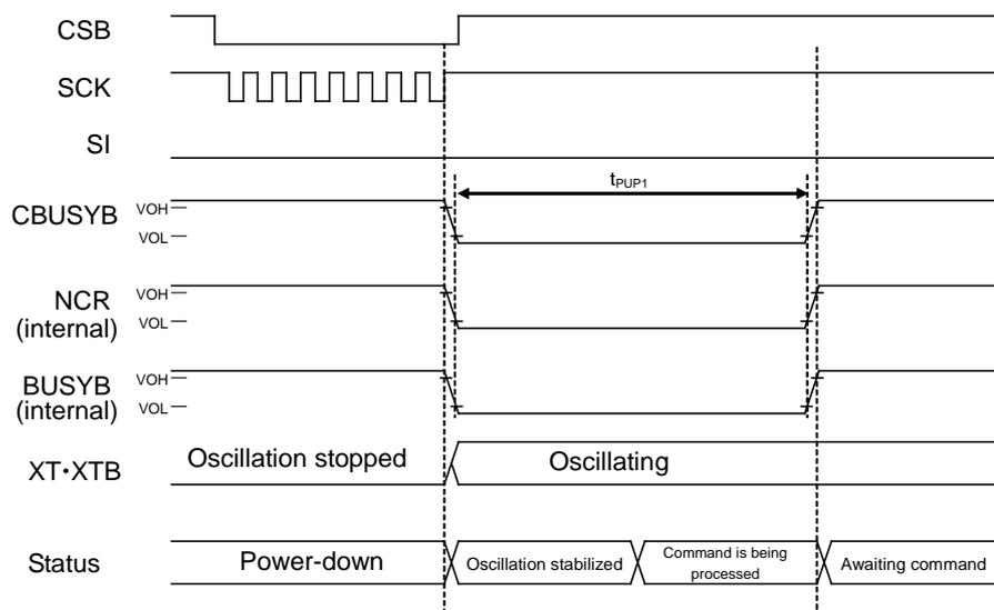
**Power-Down Timing (At the PDWN command Input)**
