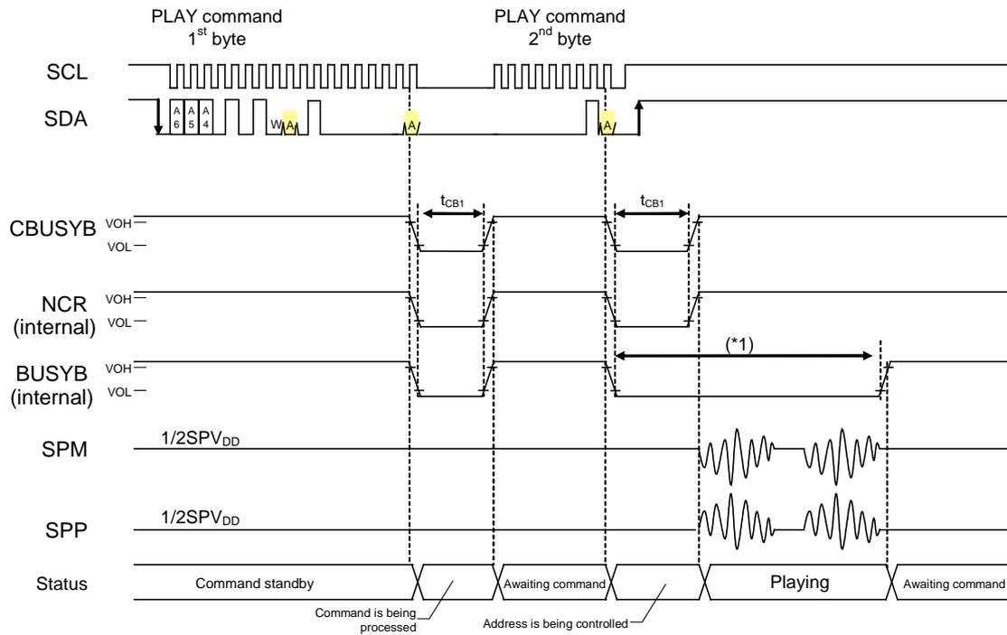
\*1: The maximum length of the “L” interval of BUSYB is  $t_{CB1} + \text{voice reproduction time} + 12\text{ms}$ .
