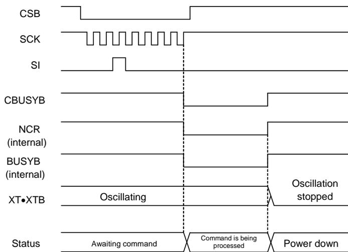
The speaker amplifier stops operation after a lapse of command processing time after the PDWN command is input. At this time, the SPM output of the speaker amplifier goes to “Hi-Z” state to prevent troubles by pop noise .
