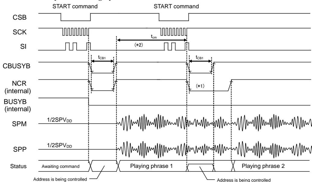
\*1: The time length of “L” level of the NCR signal during playback varies depending on the input timing of command.
