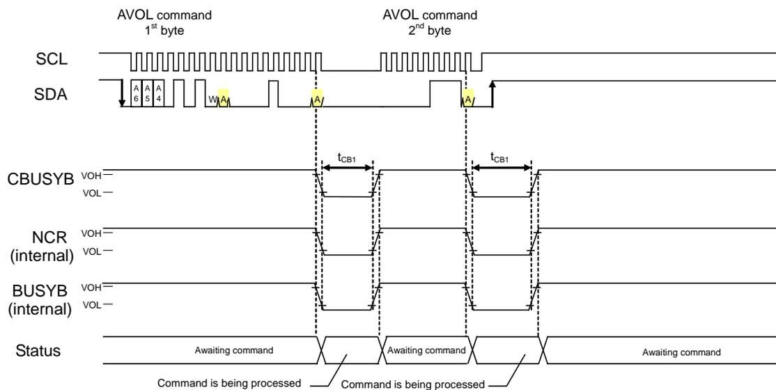
**Serial Command Interface Timing (Applied to ML22420)**
